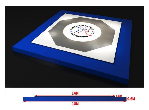
The competition venue is a square arena with a height of 0.6 meters and sides measuring 18 meters. On top of it, there is a square-shaped elastic cushion with sides measuring 14 meters and a thickness of 0.06 meters. The effective competition area is a regular octagon with a diameter of 10 meters. Beyond the octagon, there is a 2-meter-wide protective zone.
